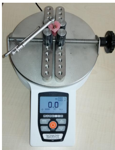
Figure 2. Biomechanical (Mark 10, NY, USA); reverse torque analysis, of the implants.
